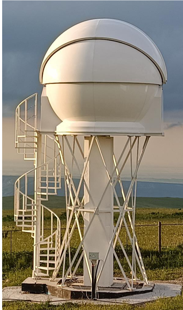
Figure 3. 4.5 m Astrosib ASD-4.5 all-sky dome installed on a 5.4 m high pier at the INASAN observatory close to Kislovodsk (Russia).
