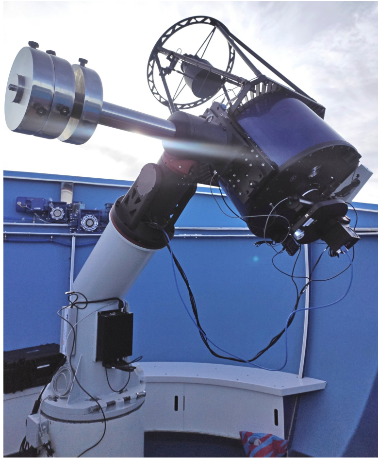
Figure 2. RC500 0.5 m aperture telescope for the second RCO station near Kislovodsk (Russia).
